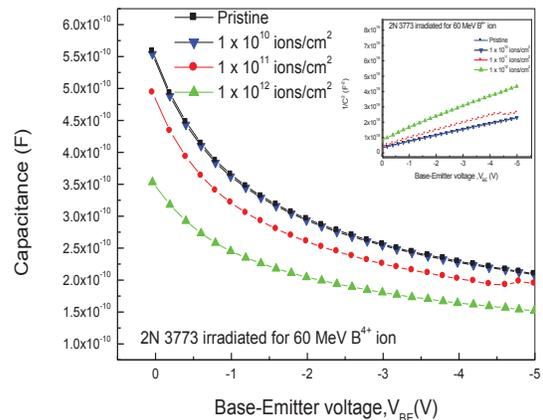
**Fig. 4:** Variation of capacitance with Base-Emitter voltage,  $V_{BE}$ . Inset shows the variation of  $(1/c^2)$  with  $V_{BE}$ .
