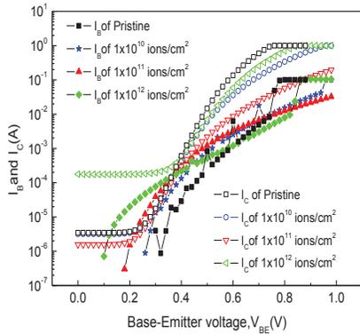
**Fig. 1:** Variation of Base current and Collector current as a function of Base-Emitter voltage with  $V_{CE} = 5\text{ V}$
