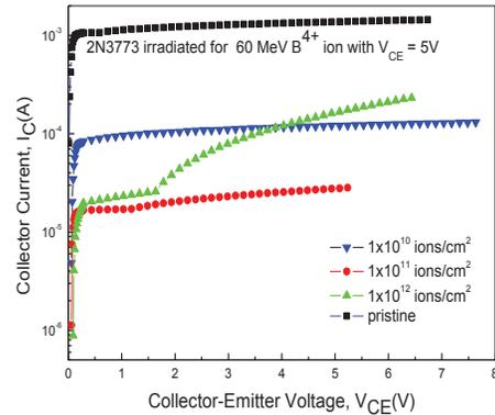
**Fig. 3:** Variation of collector current as a function of collector-emitter voltage,  $V_{CE}$  at  $I_B = 0.5\mu\text{A}$
