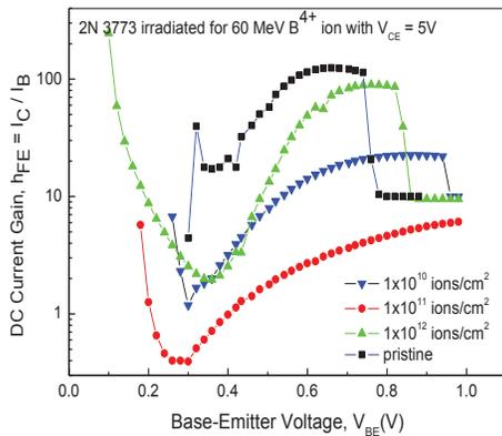
**Fig. 2:** Variation of DC current gain as a function of base emitter voltage  $V_{BE}$  at  $I_B = 0.5\mu\text{A}$
