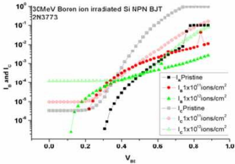
**Figure 1.** Forward gummel characteristics of 30 MeV Boron ion irradiated 2N3773 Si NPN BJTs
