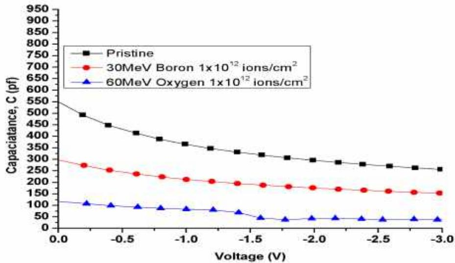
**Figure 5.** Capacitance-voltage characteristics of 30 MeV boron and 60MeV Oxygen ion irradiated 2N3773 Si NPN BJTs
