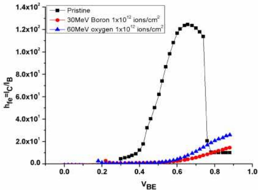
**Figure 3.** Current gain versus V<sub>BE</sub> 30 MeV boron and 60 MeV oxygen ion irradiated 2N3773 Si NPN BJTs
