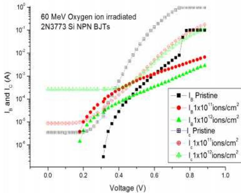
**Figure 2.** Forward gummel characteristics of 60 MeV oxygen ion irradiated 2N3773 Si NPN BJTs
