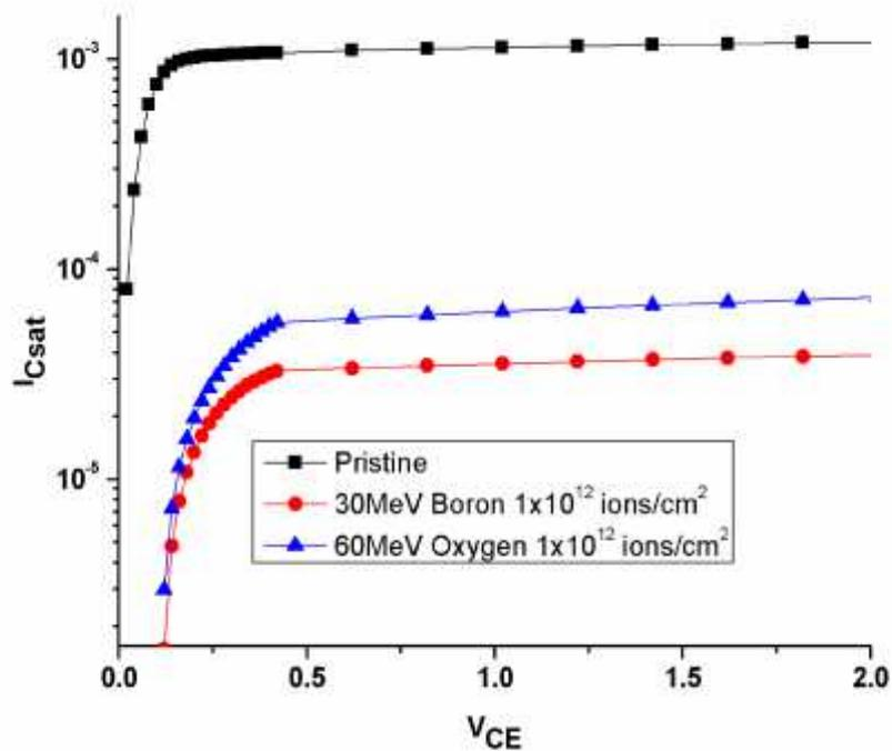
**Figure 4.** Output collector current characteristics at  $I_B = 50\mu A$  before and after 30MeV Boron and 60MeV Oxygen ion irradiated 2N3773 Si NPN BJTs
